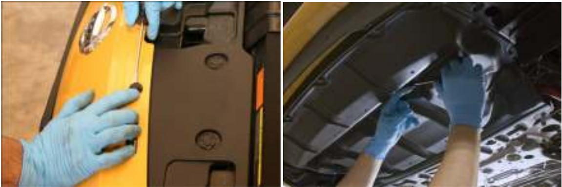
To remove the outer 2 bolts, you must pull the inner fender away from the bumper to access them. Carefully remove the front bumper and set in a safe place. Place the bolts and push pins in a safe place taking note where they came from. Then remove side panel and oil filter.
