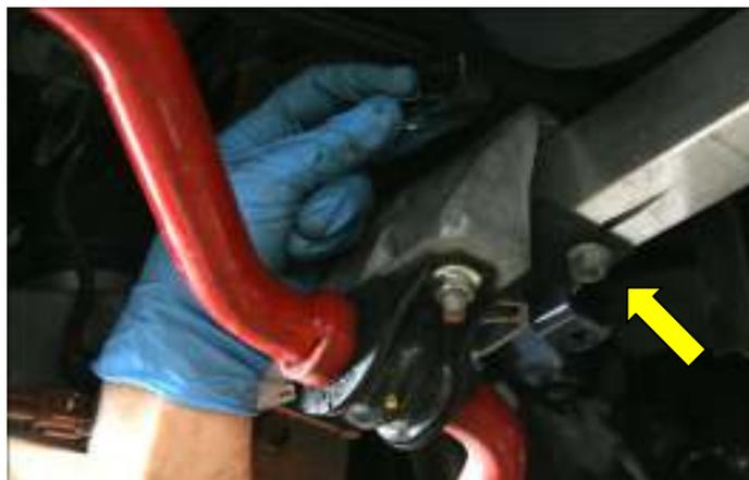
3. Hold the new oil cooler up to the cross member with fittings facing down. Lining up the end of the cooler to the end of the cross member on the driver side. Mark the slots with a felt tip pen after adjusting cooler so all four holes are on the cross member, pushed up against the frame on the back side. Remove cooler and drill holes in cross member centered in your marks with the 5mm drill bit supplied. Then carefully tap the holes with the 6x1 tap supplied.
