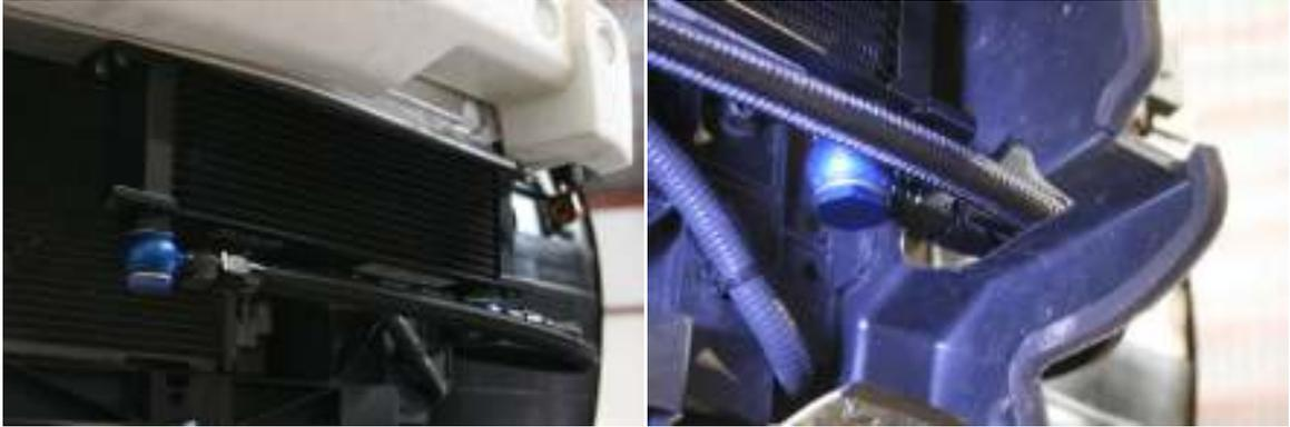
7. Install oil line separators with one at the end of the engine block, one just past the P-clamp and one where the two lines come together at the cooler.
