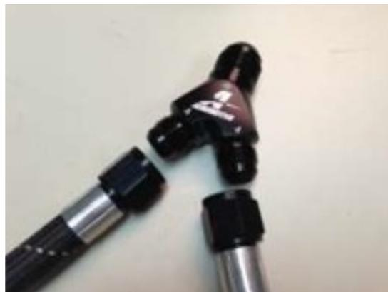
15. The other hoses attach to the rear of the rails and run to the Fuel Pressure regulator
