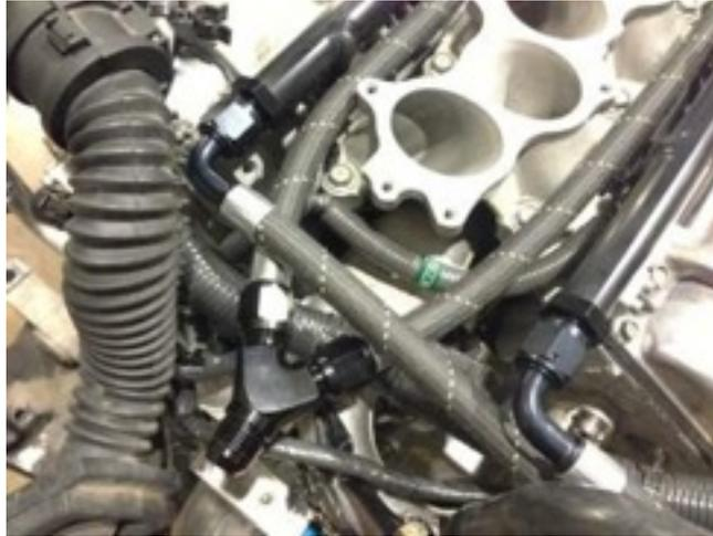
16. Run the Feed and return lines to the regulator and the y-block accordingly.
