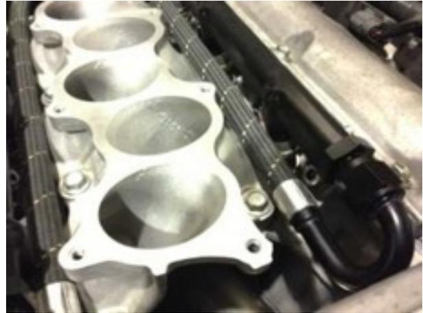
14. The Y-block attaches to at the back side of the engine to the two lines running to the front of the rails
