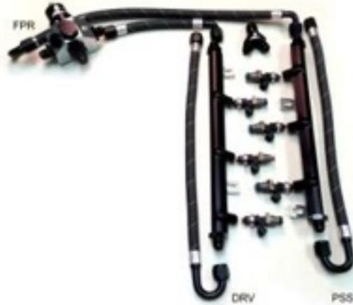
13. Install fuel rails and run the hoses on the inside of the rails. The 180 deg fittings are at the front of the engine.
