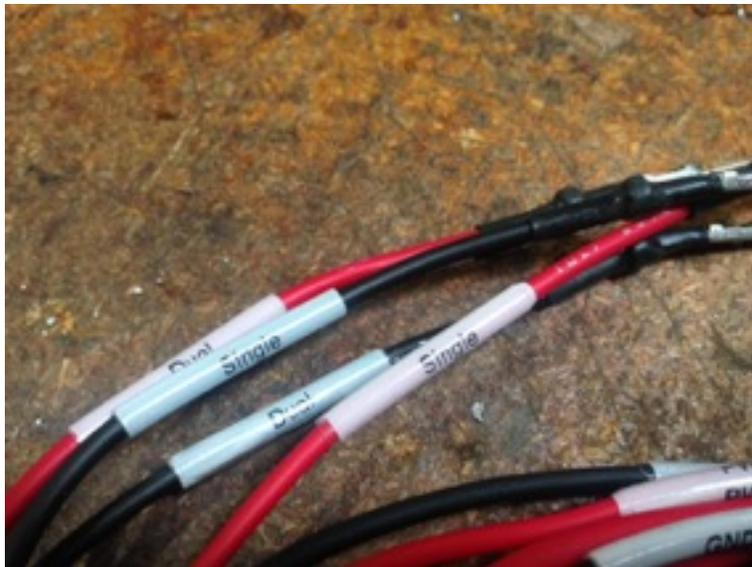
The “Single” wires activate a single pump and should be wired into primary OEM harness connector (5 pin). See diagram
