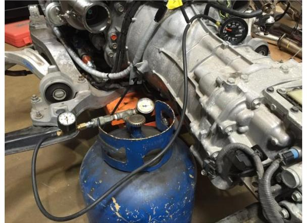
4. SLOWLY increase pressure while monitoring the wastegate flaps inside of the turbo exhaust housings. Once your targeted boost level is reached, the wastegate actuators inside of the turbo exhaust housings should open. Verify that BOTH wastegates are opening at your desired boost level.
