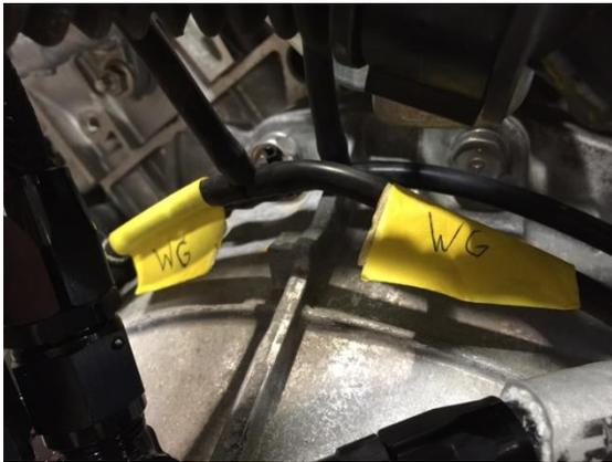
2. Locate the single vacuum line which both wastegate actuators T into.
