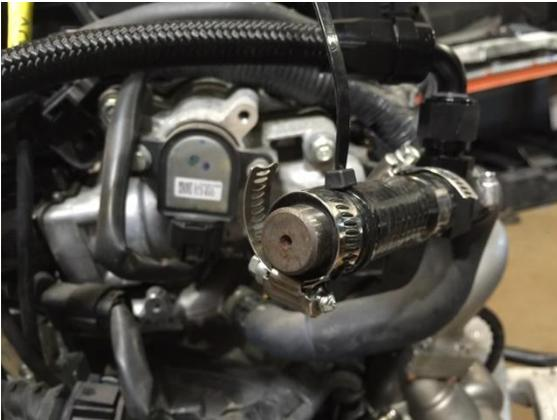
3. Verify that all plugs are and clamps fit properly, as they will need to be air tight in order to effectively hold pressure for testing purposes.
