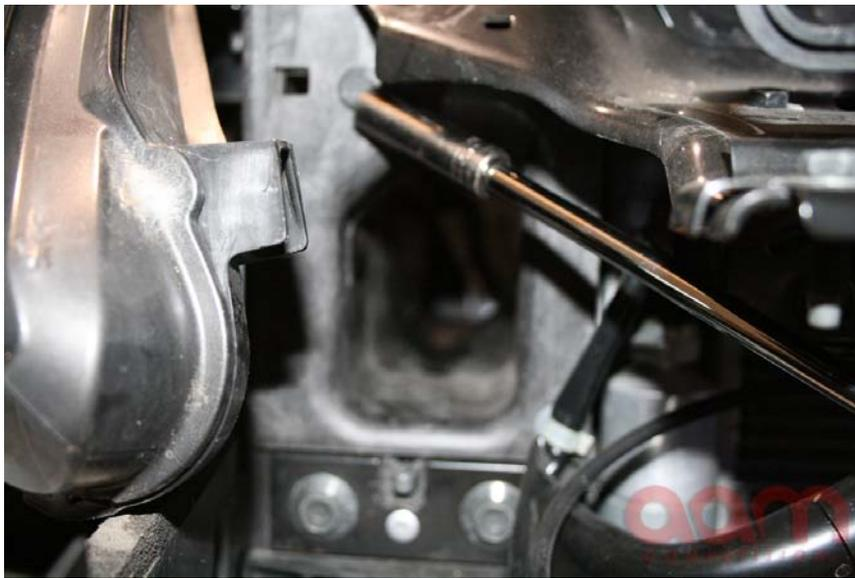
17) Using an air saw, router, grinder, dremel or any cutting tool. Open up intake air duct to fit new intake
