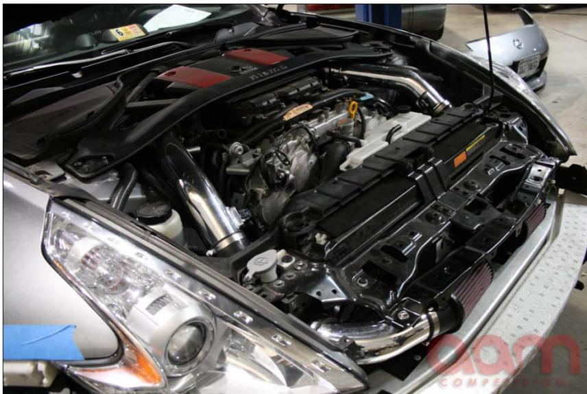
6. On the driver side, the PCV hose will clamp right onto the new intake
