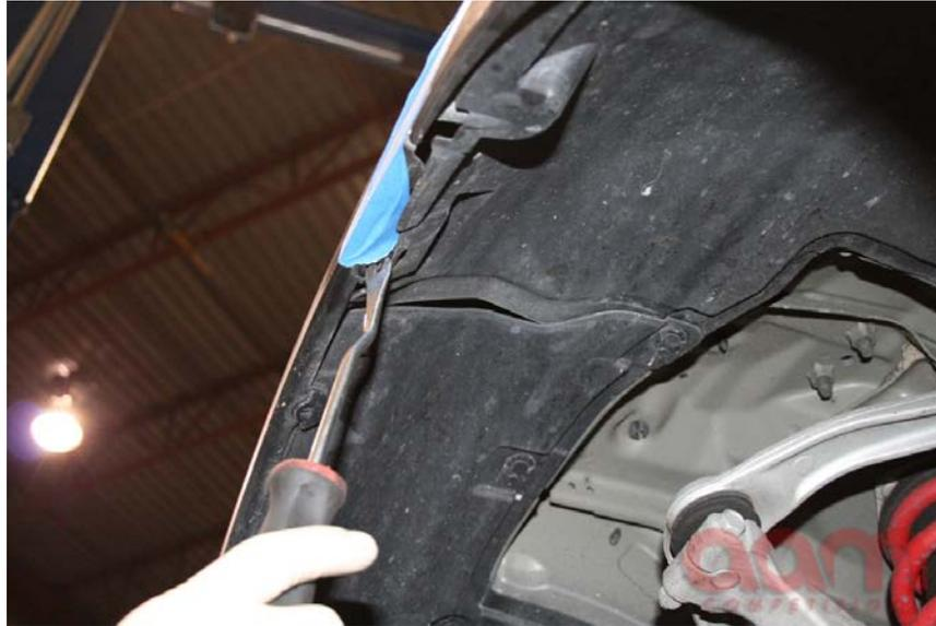
12) Remove 10mm screw securing bumper
