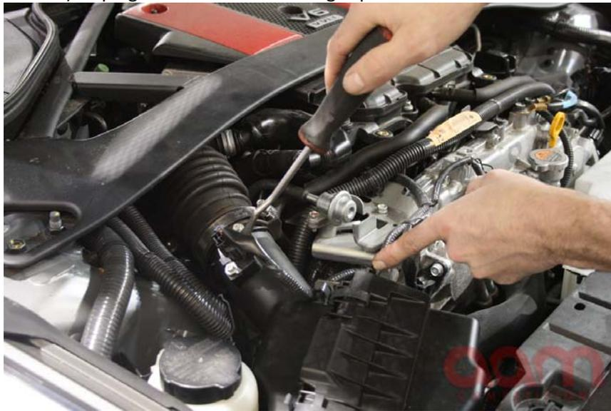
3) Loosen worm clamps at throttle bottle and air box, remove intake boot
