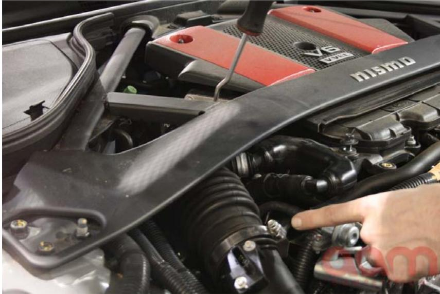
5) Remove 10mm bolt securing airbox
