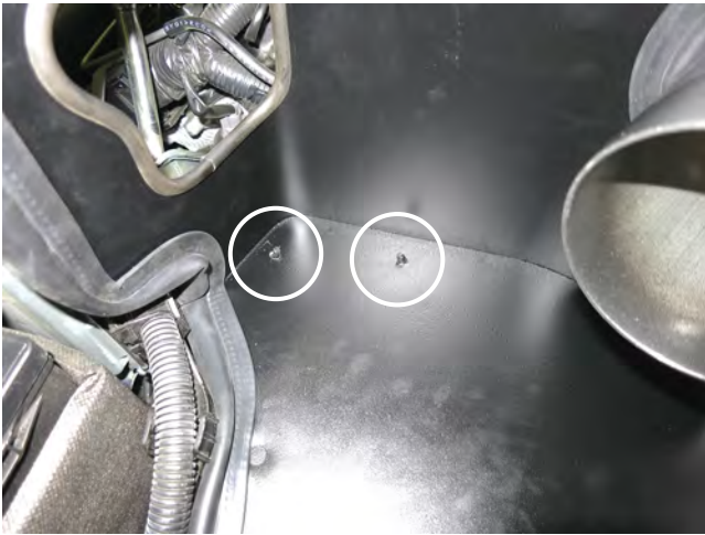
i. Install the transmission vent line clips to the heat shield from the bottom.
