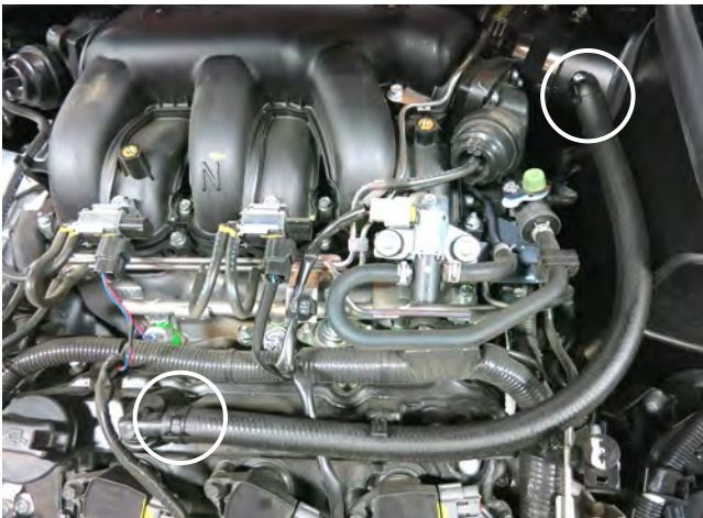
k. Install the completed vent line onto the AEM intake tube and the 90° fitting. Then, secure with the spring clamps.
