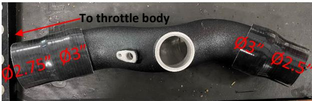
9. Install the AAMC recirculation tubes using the supplied worm drive clamps.
