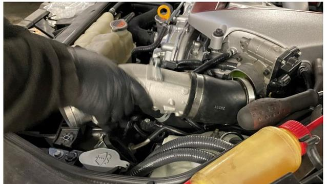
7. Remove the stock recirculation tubes using pliers to loosen the clamps on the tubes.
