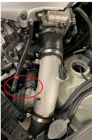
5. Loosen all the clamps shown below to remove the upper intercooler pipes.
