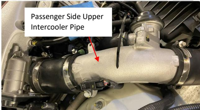
4. Disconnect the vacuum line and hose going into the stock blow-off valves on the upper intercooler pipes. Use pliers to remove the clamps.
