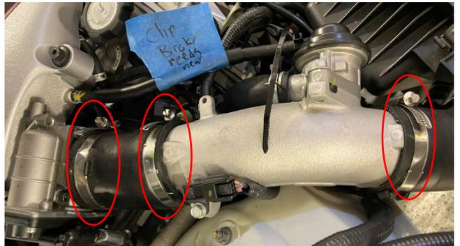
6. Once all clamps have been loosened, remove both upper intercooler pipes along with the throttle body couplers attached to both ends of the pipe.
