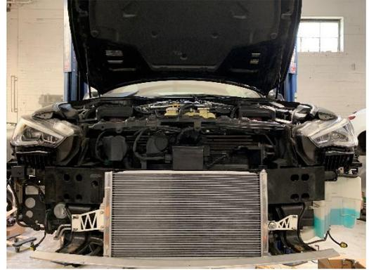
**23.** Attach the short 90° hose to the metal hose sleeve and the lower port of the AAM Competition Heat Exchanger using the OEM hose clamps. **For Redsport models or vehicles with a second auxiliary fluid pump, use the hose on the outlet side of the pump, which can be rotated down and attached using the 90° hose fitting.**
