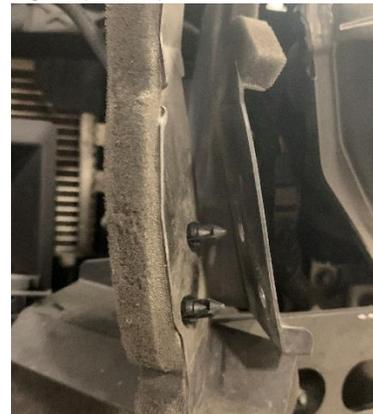
**12.** Use a 12mm socket and a 12mm wrench to remove the fasteners on each side of the crash beam, leaving one per side to keep the beam steady.
