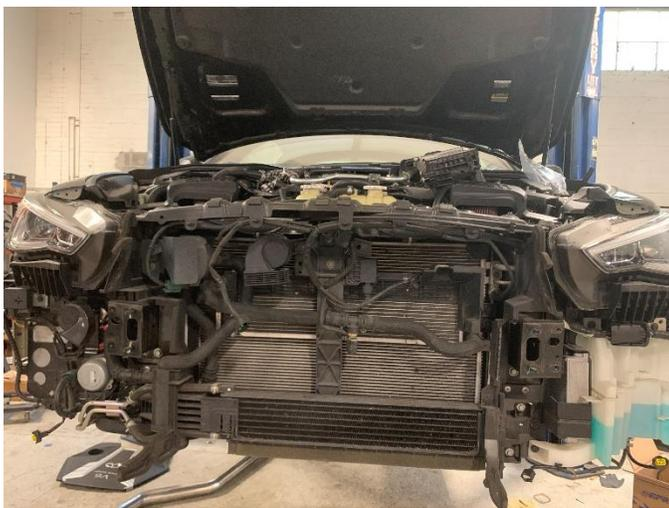
**15.** Remove the bolts from the oil cooler, then use zip ties to keep it out of the way.
