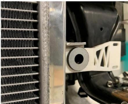
**22.** Position the heat exchanger behind the aluminum bumper brace and in front of the crash support using the remaining M6 hardware for the mounts, and the M8 hardware through the grommet.
