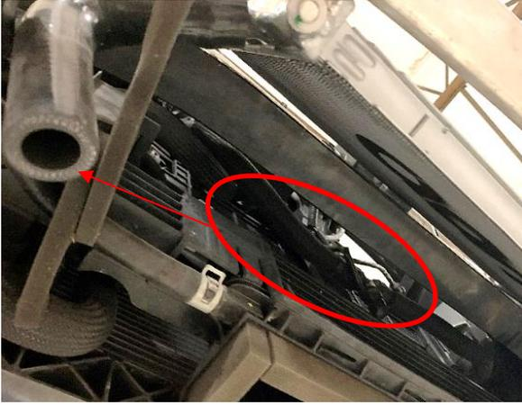
**24.** Attach the long hose to the T-fitting and to the driver's side port on the AAM Heat Exchanger.
