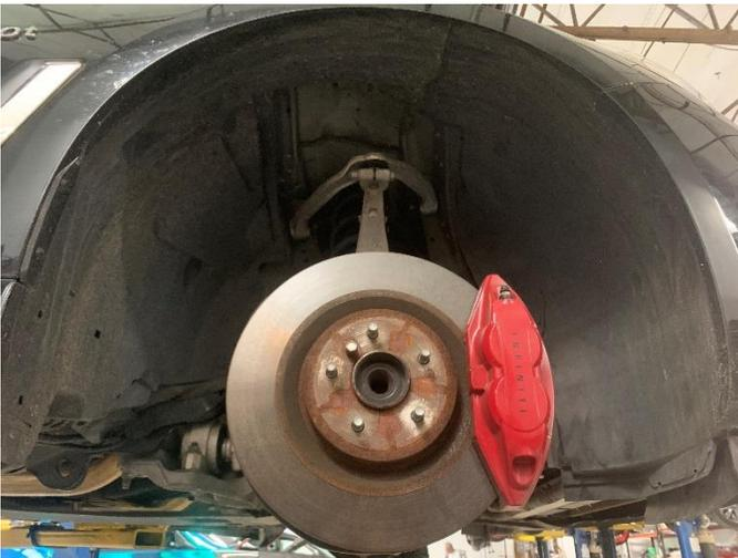
4. Remove the wheel well liners on each side by disconnecting all push clips.
