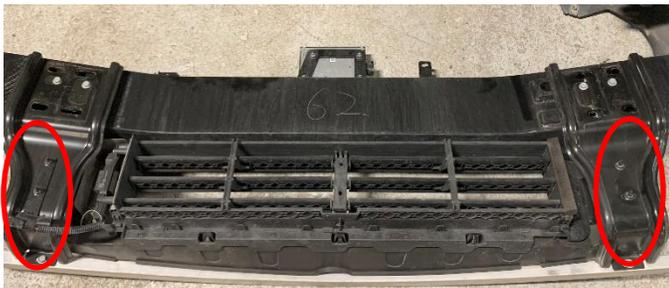
**14.** Prop up the crash beam so that it will not fall, then remove the last bolts from each side. Store in a safe place.
