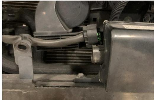
11. Disassemble the trim shrouding near the crash beam by disconnecting the push clips.
