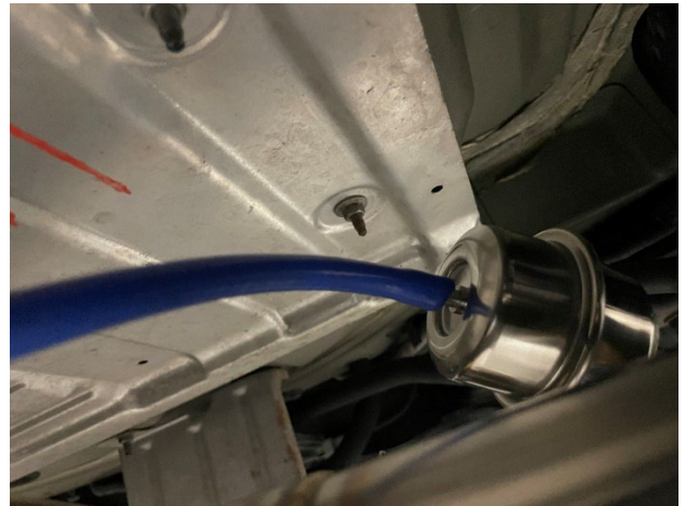
23. Route the vacuum lines from the vacuum tee to the valve actuators on each side as shown below.
