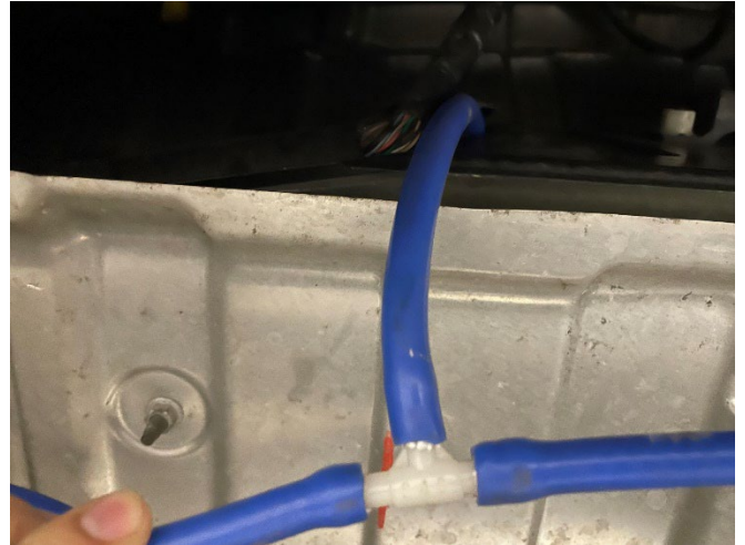
23. Route the vacuum lines from the vacuum tee to the valve actuators on each side as shown below.
