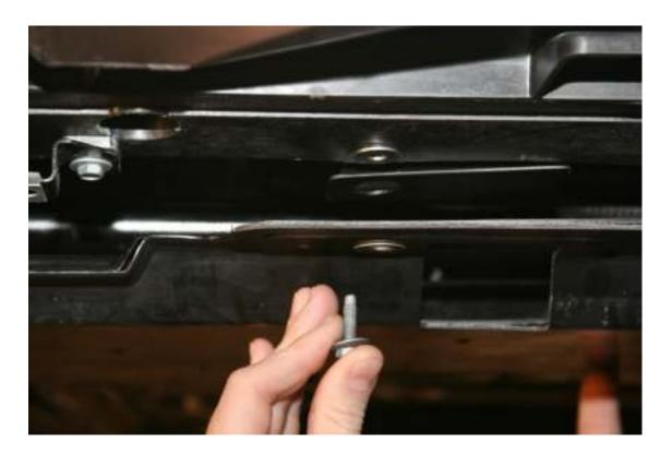
o. If there are no leaks, you can now begin to reinstall the belly pans, inner fender, wheel and top engine cover. The oversized washer will be discarded now as the mid-pan goes up first. The bolt that holds the pan up here will hold the bracket in place as well.
