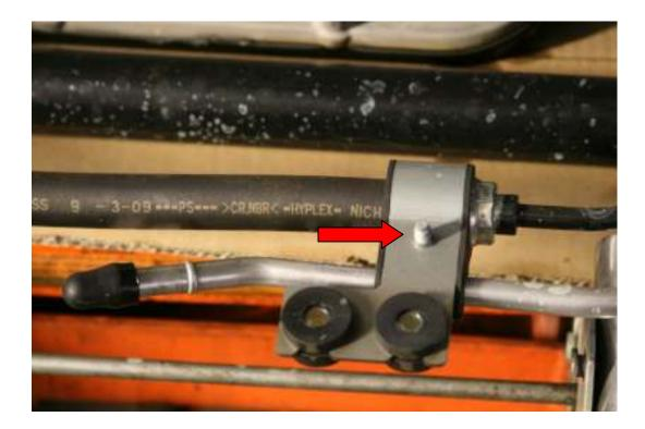
f. Remove the 6mm bolt that's clamping the two power steering lines together and set aside. You will be reusing this later. Then remove the two bolts holding this clamp to the radiator support. You must then drill out the single hole with a 5/16" bit to get rid of the threads. Deburr the hole and set aside for now.
